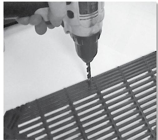
6. Once the new holes are drilled into the AeroFlap®, position into your bracket and secure following manufacturers instructions.
