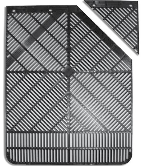
4. After the AeroFlap® is cut, place into the bracket and mark the locations of the holes.
