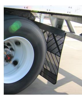
Designed for fuel-efficiency and safety, the AeroFlap's innovative design breaks up the trailing air vortex to reduce vehicle drag and reduce spray (old style shown).
